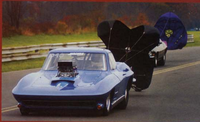
For this class, NHRA requires parachutes to stop cars capable of such high speeds. Quarter-mile times are in the 6-second range.
