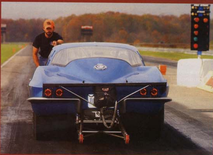
The rear split-window has been removed to increase visibility when backing up after a tire-heating burnout. Knowledgeable crewmembers are helpful at this point to ensure the car is positioned properly.
