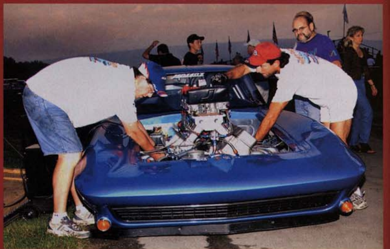
The huge 472ci small-block Chevrolet engine makes nearly 1,300 hp on nitrous oxide, 900 without. Note the custom sheetmetal intake-manifold system.
